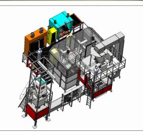
Automatic stations for fitting the bottom bars on positive plates:
